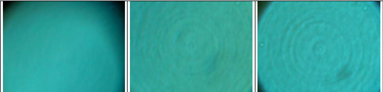
Fig. 2 - 4. The circles and bubbles photographed through 3 different Pentax-objectives f = 18, 24 , and 50 mm. The microscope-objective was removed from the revolver (nosepiece), and the Pentax-objective was placed on a microslide and then centered.
